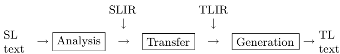
Fig. 1. Main structure of an (indirect) rule-based transfer MT system. Source language (SL) text is analyzed and converted into an intermediate representation (SLIR), then transformations are applied giving as a result a target language intermediate representation (TLIR), finally the TLIR is used to generate the output translation into the target language (TL).
